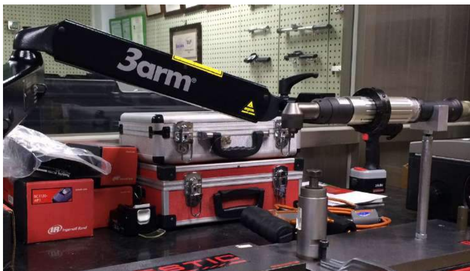
A compact multi-purpose arm for use when brakes are not required
