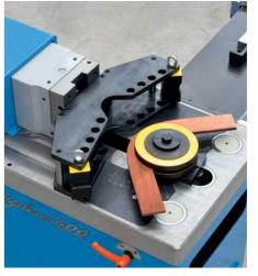
2 jaw bending tool with set of flanges for flat and shaped bars up to 90°. Max 60 x 20 mm.
