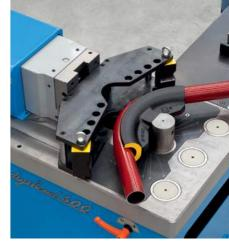
2 jaw bending tool for thick wall pipes from 3/8" gas (17.2 mm) up to 2" gas (60.3 mm) and round bars, up to 90°.
