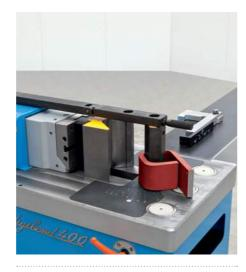
Pin bending punch Ø 80 mm with antiflexion bar for bending a closed loop into thick wall bars. Max 200 x 15 mm.
