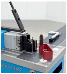
Bending tool with pin Ø 50 mm, H=200 mm, revolving pin single V die and antiflection bar. max. 200 x 8 mm.
