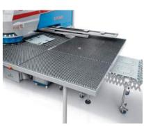
In combination with machines with side chute door, two additional unloading points are provided: 1) up to max part size 200x200 mm 2) up to max part size 1500x1000 mm depending on machine throat size.
